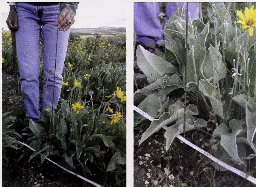
Figure B-2. Measuring plant species using the line-point intercept technique (pin size exaggerated to emphasize method).
