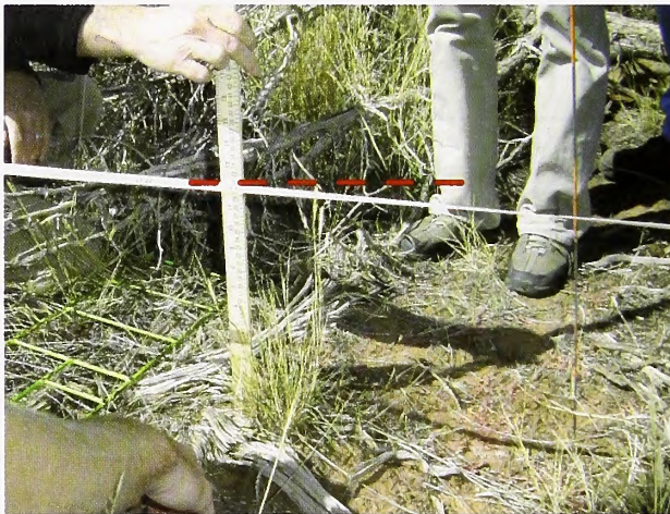
Figure B-3. Grass and forb height measurements. Record natural or "droop" height of grasses and forbs. Note the dashed red reference line.
